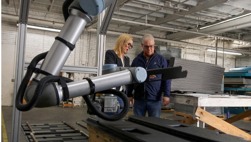
Caption: CEO Juliet Oehler Goff and outside consultant Dan Sproles inspect finished parts as the cobot finishes trimming. The cobot offers high accuracy and consistency, and has helped reduce late shipments to under one percent.
