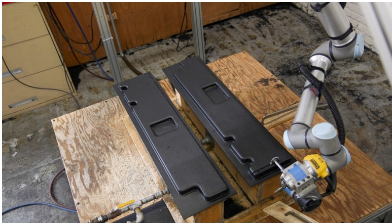
Caption: The extended reach of the UR10e cobot, which is top-mounted on a gantry, means it can trim two parts per setup, cutting trimming time nearly in half compared to previous manual trimming.
